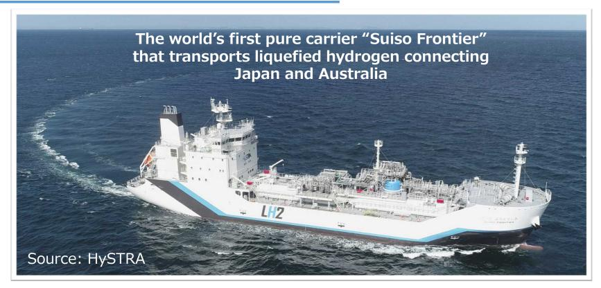
Electrical propulsion ship with a total length of 116 m, cargo tank capacity of 1,250 m<sup>3</sup>
