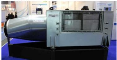
SCR (a selective catalytic reduction device)
