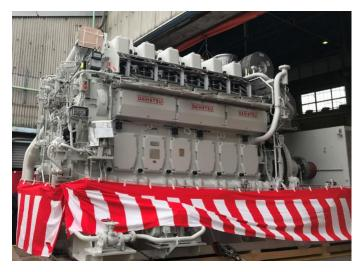
First dual fuel engine for JAXA (continuous/emergency power generation)
