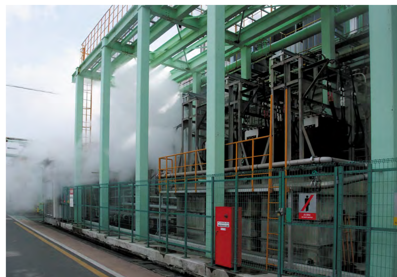
試験運転時、水負荷槽から発生する多量の蒸気 Large amounts of steam being generated from the water resistance load tank during test operation.
